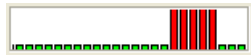
Figure 7.4. Miniature Ping View displaying successful Ping packets (green) vs. lost packets (red).
